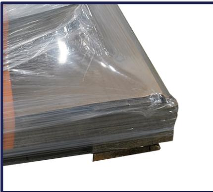
Shrinkwrap to pallet, with wrap extending down around pallet as well as the battery. Make sure enough wrap is used to prevent easy tearing of the wrap.
