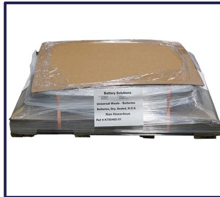
Attach appropriate labels to outermost layer of shrink wrap or packing material.
