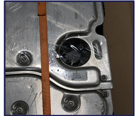
Make sure orange plug is removed and area is protected from contact.
